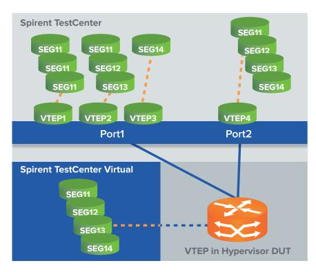
Using Spirent's Topology Emulation, the VXLAN VTEP and VMs that are emulated have the capability of running any of Spirent TestCenter protocols (including application layer: HTTP, FTP, Video) over a fully encapsulated VXLAN segment. This will quickly find the capacity and forwarding rate of any VTEP, VTEP Gateway, switch, firewall or forwarding device supporting VXLANs.
